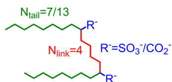
Figure 1. Gemini-surfactants utilized in this work. For example, nomenclature \text{SO}_3\text{-}13(4) denotes a gemini surfactant with sulfonate headgroups, 13 carbon atoms constituting each tail, and four linker carbon atoms.
